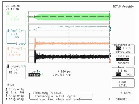
Figure 1 – Analyzing the keying envelope and frequency stability of a gated oscillator
